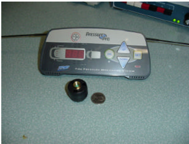
This picture shows the receiver / monitor and one sensor compared to a Canadian nickel coin.
